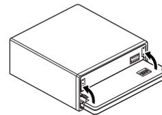
4. Fix the front panel to the unit using screws.
