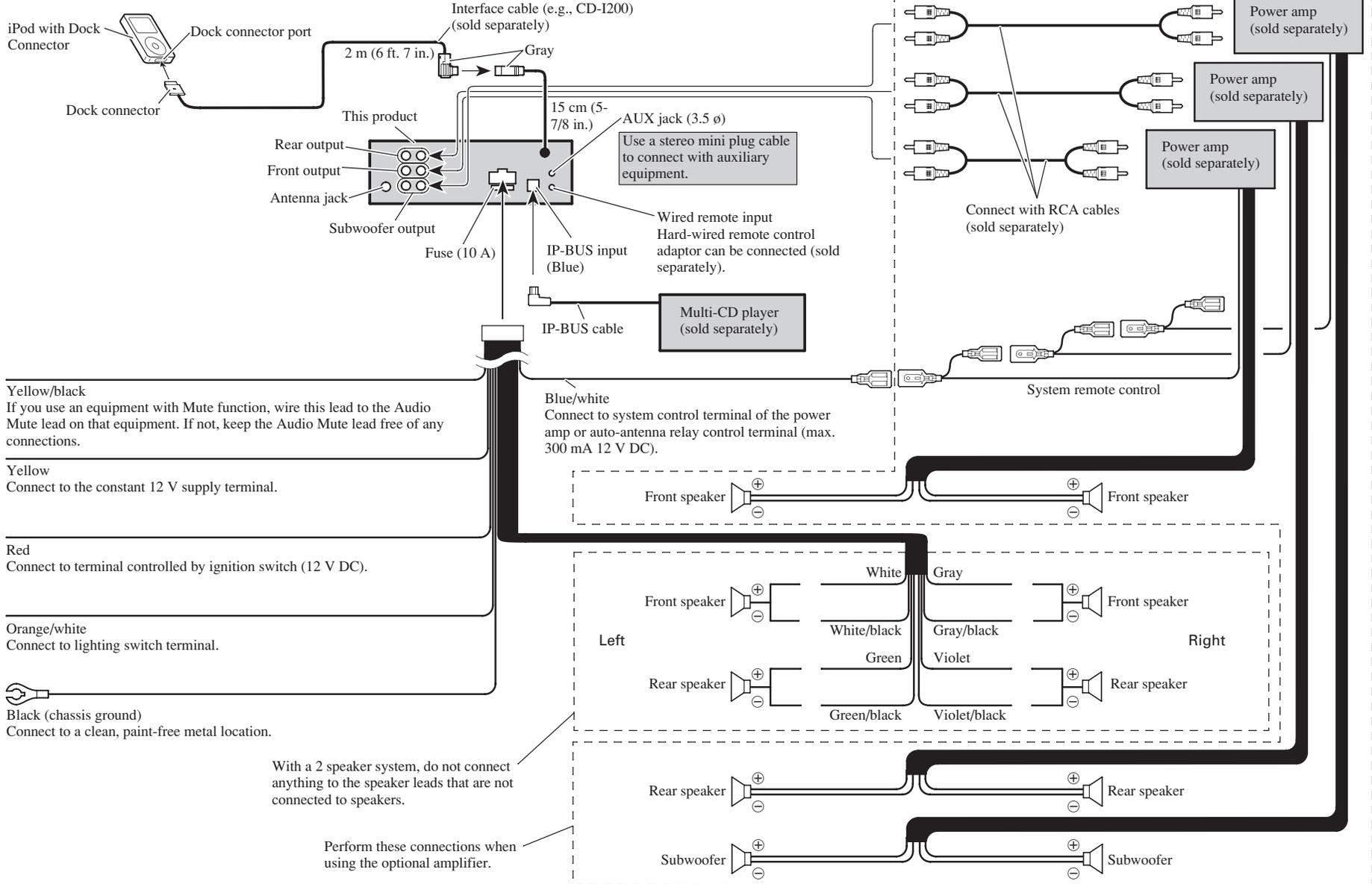
When using a Subwoofer without using the optional amplifier
