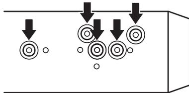
3. Tighten two screws on each side.
