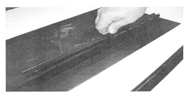
STEP 16: PLACE SLIDERAIL IN CORRECT POSITION AND PRESS DOWN FIRMLY TO SEAT
