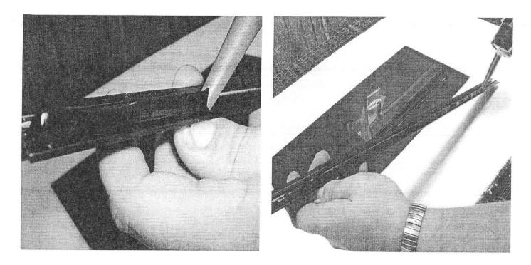
STEP 17: APPLY URETHANE TO HINGE AS SHOWN IN THE ABOVE TWO PICTURES
