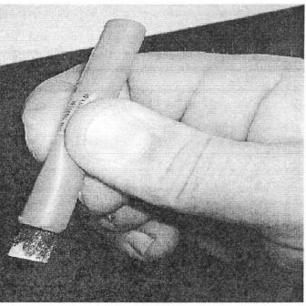
STEP 7: YOU WILL NEED TO ACTIVATE THE PRIMER PEN... DO THIS BY PINCHING IN THE MIDDLE OF THE PEN LIKE SHOWN IN THE LEFT PICTURE... ALLOW COMPOUND TO COVER ENTIRE FELT TIP
