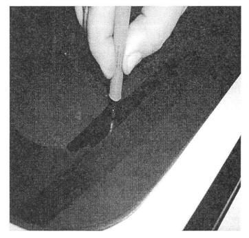
STEP 8: APPLY PRIMER TO GLASS ONLY ON TOP OF AKTIVATOR AREA ONLY IF SLIDERAIL WILL NOT BE COVERED BY EXISTING SILKSCREEN ON GLASS
