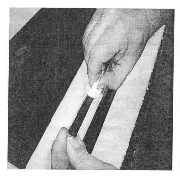
**STEP 10**: APPLY AKTIVATOR PAD AS SHOWN ABOVE TO SLIDERAIL SECTION TO BE URETHANED
