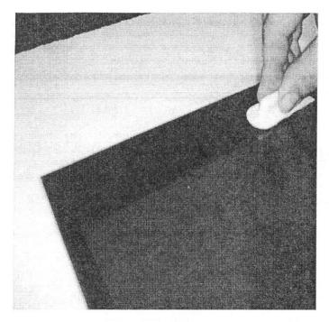
STEP 3: APPLY AKTIVATOR PAD AS SHOWN ABOVE TO ONE SECTION AT A TIME THAT WILL HAVE URETHANE APPLIED
