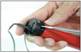
Separate the Collar on the new motor and slip it down over the motor tube.
