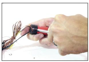
4 Locate where the Collar is separated and, with a flat-bladed screwdriver, gently pry it open allowing it to slip over the motor tube.
