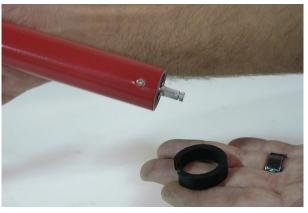
**6** Collar removed from the motor assembly.
