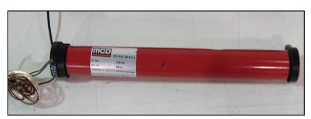
**15** Completed Motor. Insert in shade roller tube.
