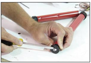
**14** Replace the E-clip to hold the External Drive Gear in place.
