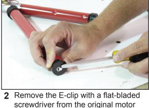
screwdriver from the original motor assembly.
