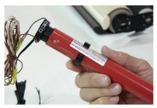
Slide the old Collar onto the new Motor and snap it in place in the upper groove.
