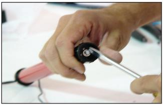
**7** On the new motor, remove the External Drive Gear by removing the E-clip and sliding the Gear off the shaft.
