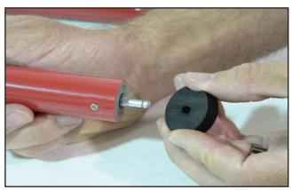
**13** Take the original External Drive Gear and place on the new Motor shaft.
