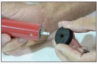
Slide the External Drive Gear off the shaft.
