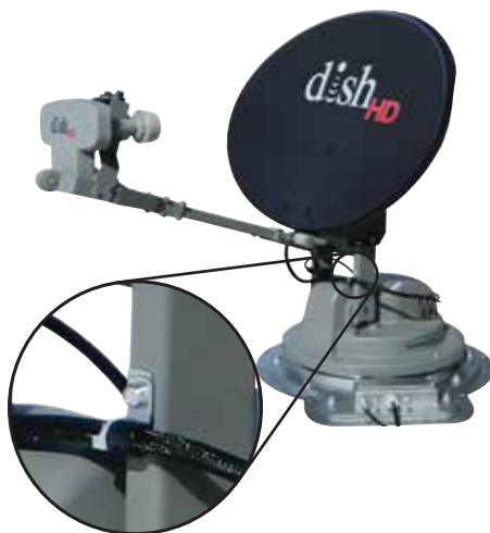
P-clamp installed 14" from ends of sheathed cables, next to zip tie on sheathed cables
