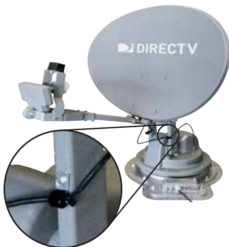
P-clamp installed 14" from ends of sheathed cable, next to zip tie on sheathed cable
