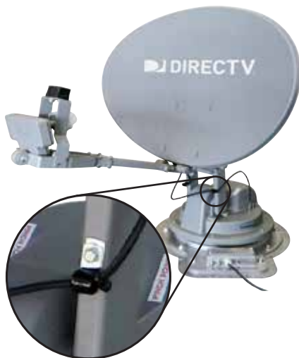
P-clamp installed 14" from ends of sheathed cables, next to zip tie on sheathed cables
