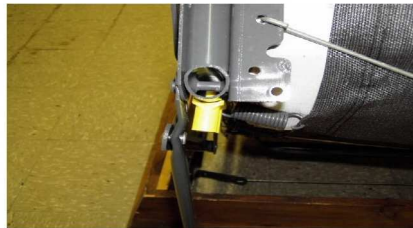
4. Styling block should be flush with bottom of tube when finished.
