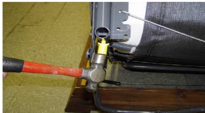
3. Tap lightly with hammer until shaft is completely inserted into tube.
