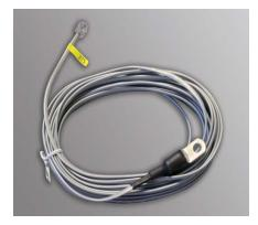
A plug-in external Battery Temperature Sensor (BTS) is provided for units with the battery charger feature. When installed, the BTS automatically adjusts the battery chargers BULK, ABSORB and FLOAT voltage setpoints based on temperature. If the temperature sensor is NOT installed and if the batteries are subjected to large temperature changes, the battery life may be shortened.
