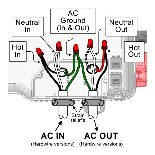
Figure 11, AC Wiring Connections
