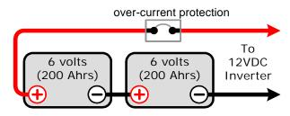
12 volt battery bank (total capacity = 200 Ahrs)
