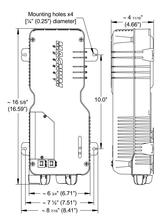
Figure 8, MM Series Inverter Dimensions
