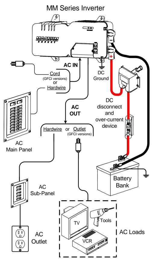
Figure 6, Basic Installation Diagram
