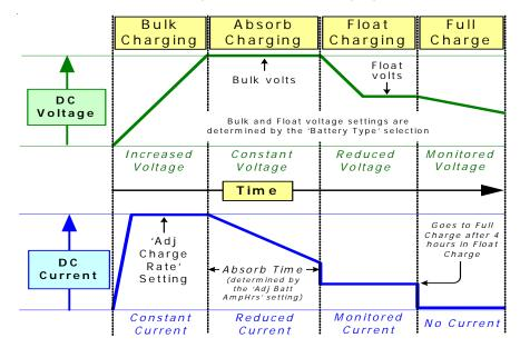
Figure 12, Automatic 4-Stage Charging Graph
