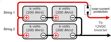
12 volt battery bank (total capacity = 400 Ahrs)
