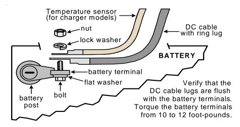
Figure 9, DC Cable to Battery Terminals
