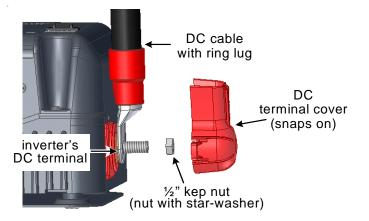
Figure 10, DC Cable to Inverter's DC Terminals
