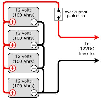
12 volt battery bank (total capacity = 400 Ahrs)
