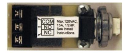
The Relay Module can be used to safely control (on/off) any 120V appliance using 12V signals. The Relay Module is just a simple SPDT relay that has been repackaged, having both Normally Closed (NC) and Normally Open (NO) contacts available through screw terminals. With the Common (COM) and NC contact, connected to a TV, Block Heater or Awning, it can be used as an Ignition Lock-out feature. Using the NO and COM contacts, the Relay module can control a Water Heater.
