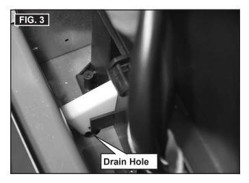
4. Slide spout into position making sure the back edge is inside the drain hole. See FIG. 3.
