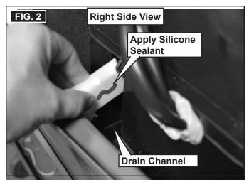
3. Apply a small amount of silicone sealant to each side of the right (longer of the two) spout. See FIG. 2.
