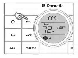
Press the ZONE button to cycle through the available zones to be programmed. Each zone signifies a unit designated to cool, heat or dehumidify a specific area of an RV. The Dometic CCC 2 thermostat can control up to four units (zones).
