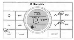
6. Press the CLOCK button to initiate the clock setting sub-menu on the CCC 2 thermostat. When entering this menu, the "hour" digits will flash first. Press the CLOCK button again and the "minutes" digits will flash. Press it a third time and the "AM" or "PM" icon will flash. Press the UP ∧ and DOWN ∨ buttons to set the "hour", "minute", and "AM/PM" setting.
