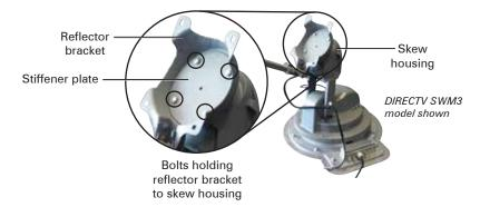
6 Remove the LNB arm assembly, and set aside; you will need this assembly later.
