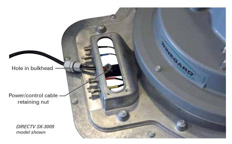
**3** Thread the washer, and tighten.
