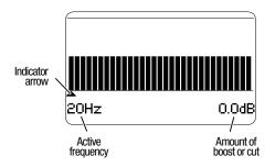
The arrow indicates the selected band; the band s center frequency is indicated on the left side of the screen; the amount of boost or cut that you apply is indicated on the right side of the screen.
