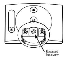
b) Select one of the other two viewing-angle positions. Reassemble the parts in reverse order and tighten the recessed hex screw.
