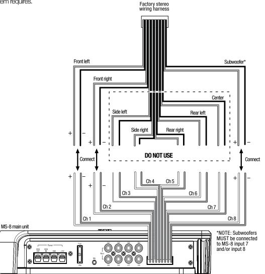
NOTE: The above illustration shows only a general connection example and does not represent any particular vehicle audio system.
