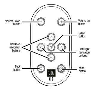
**Volume Up and Down buttons:** Pressing either of these buttons at any time (except during the setup/calibration process) will display the MS-8's **System Volume** screen, allowing you to change the audio volume. The volume range is between –80dB and 0dB.
