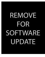
After downloading a firmware upgrade into your PC, remove the sticker and connect the Update port to a USB port on your PC. Follow the directions that accompany the upgraded firmware to upload the new firmware from your PC to the MS-8.
