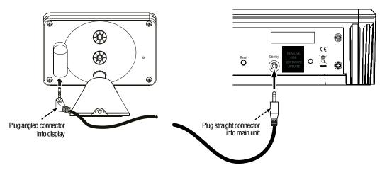
NOTE: The display unit must be connected during setup but may be disconnected after setup and after you ve made any additional adjustments in the Audio Controls menu (see *Audio Controls Menu*, on page 36). If the display unit is disconnected after setup and final adjustment, you will not be able to make any additional MS-8 adjustments, and the remote control will not function. See *Main Menu*, on page 35.
