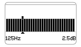
IMPORTANT: The MS-8 s digital volume and equalization work differently than standard analog controls. Boosting the MS-8 s subwoofer-level control, bass-tone control and the low bass bands in the 31-band EQ to their near-maximum, and setting the MS-8's System Volume control to 0dB, will cause severe clipping (distorted sound) that may damage your system s loudspeakers.
