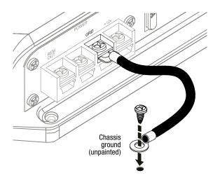
2. **+12V:** Connect this terminal to the vehicle battery s positive (+) terminal. Insert a 25A fuse in series on the +12V wire no further than 18 inches (46cm) from the battery terminal.
