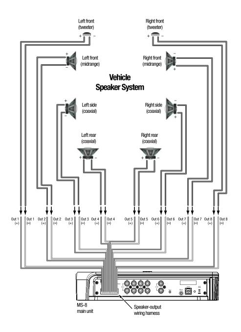
To ensure proper polarity, connect each MS-8 positive (+) terminal to the respective + terminal on the speaker. Connect the negative () terminals in a similar way.
