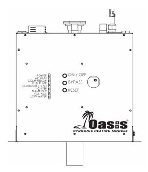
Figure 8-2 Heating Module Main Control Panel
