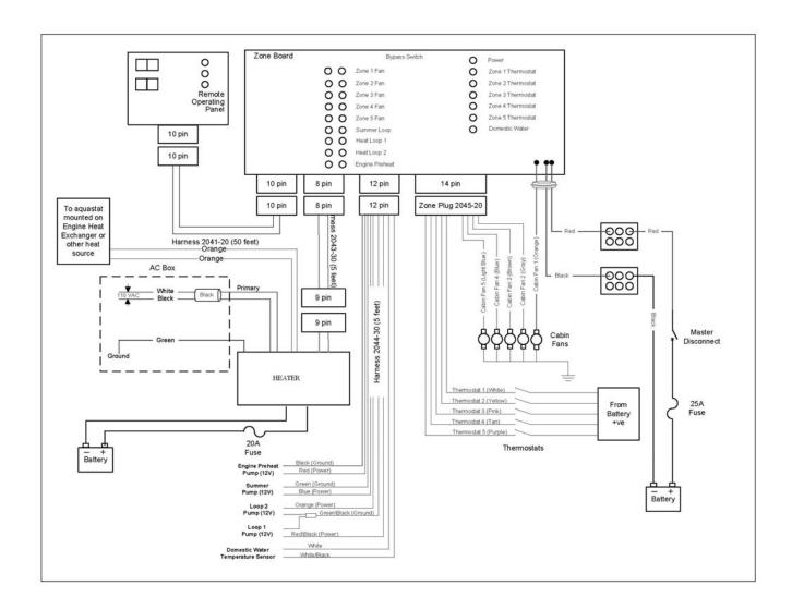
Figure 9-10: Zone Board Wiring (No DM12)
