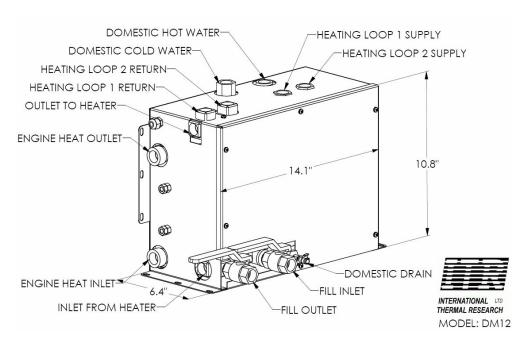
Figure 9-3: Distribution Module Fittings Location.
