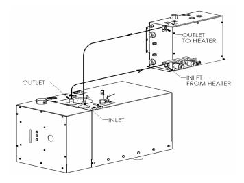
Figure 9-6: Connecting to the OASIS Heating Module
