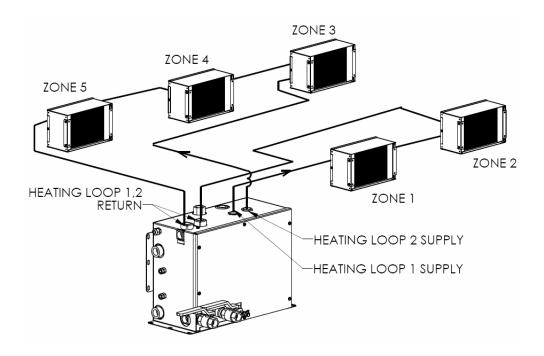
Figure 9-7: Connecting two Heating loops.
