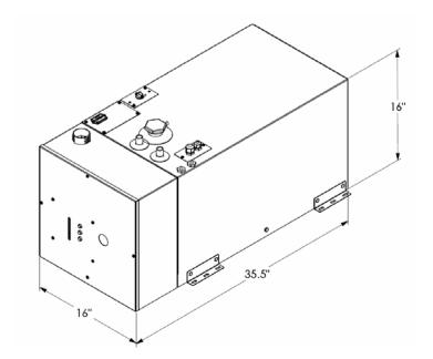
Figure 2-1: Module Dimensions
