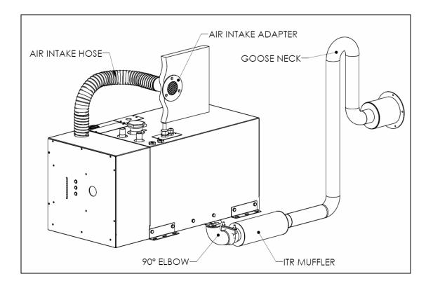
Figure 3-3: The Exhaust Goose Neck configuration
