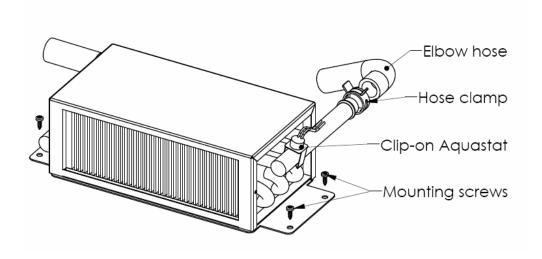
Figure 5-2: Mounting a Spacesaver Fan
