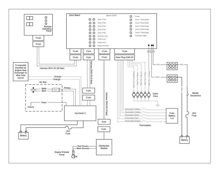
Figure 9-9: Distribution Module Wiring
