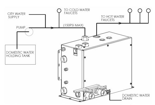
Figure 9-4 Domestic Hot Water System Plumbing.
