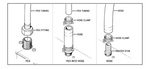
Figure 7-2: Three Approved Methods of Installing Heater Hose (consult ITR for alternative methods and products)
