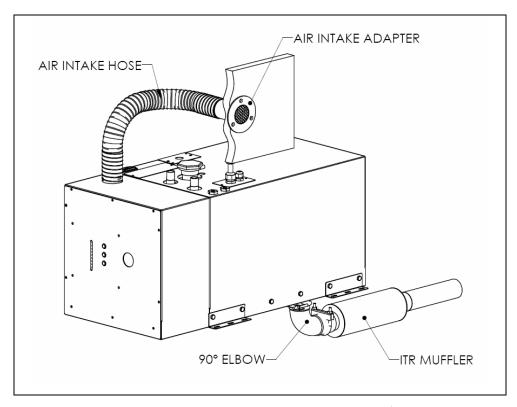
Figure 3-1: Installing the Exhaust System (Bottom Exhaust)
