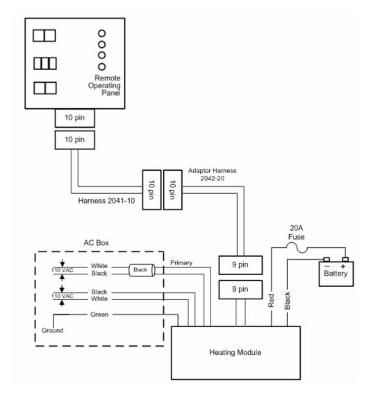
Figure 6-1 System wiring
