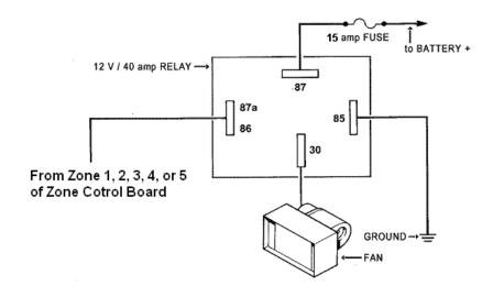
Figure 5-3: Installing a Relay for Additional Fan Amperage
