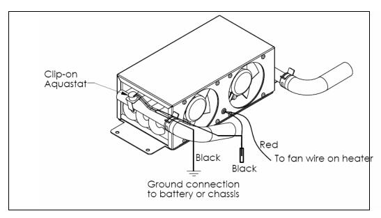
Figure 5-1: Wiring the Fan's Aquastat
