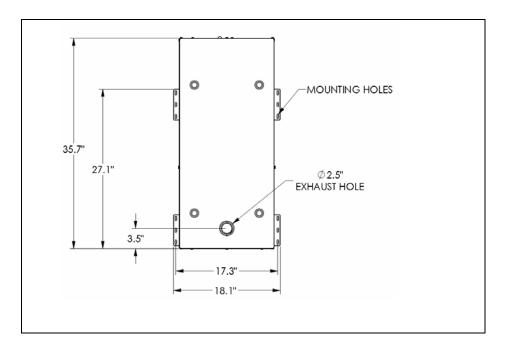
Figure 3-2: The Exhaust Hole Location & Mounting Template
