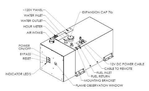
Figure 8-1 Oasis™ Heating Module
