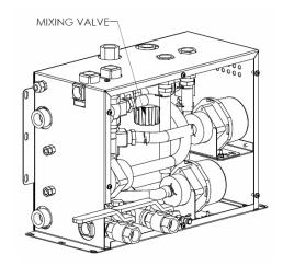
Figure 9-11: Mixing valve location
