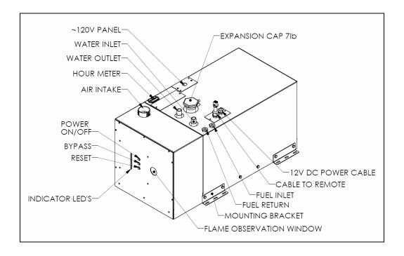
Figure 7-1 Heating Module
