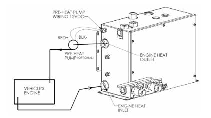
Figure 9-5 Engine Heat / Pre-heat System Plumbing.
