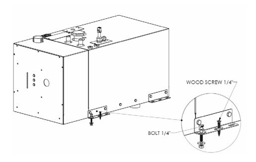
**Figure 2-2: Module Mounting Brackets**
