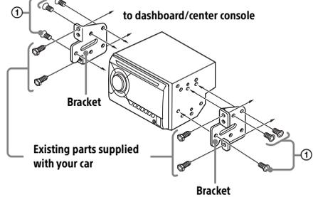
When mounting this unit to the preinstalled brackets of your car, use the supplied screws ① in the appropriate screw holes, based on your car: T for TOYOTA, M for MITSUBISHI and N for NISSAN.
