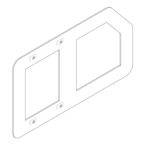
5/16 DIA. (4-PLCS) 1/4" LOW-PROFILE NARROW-BASE WELD NUT (4-PLCS) McMASTER PART #98001A135
