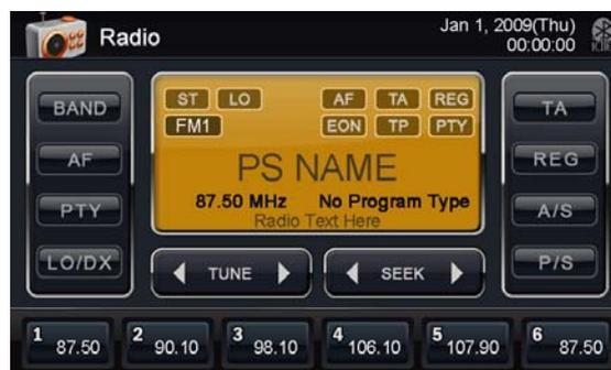
**BAND** This button allows the selection between the FM and AM bands. There are 3 FM and 2 AM ranges available, all with 6 available presets.
