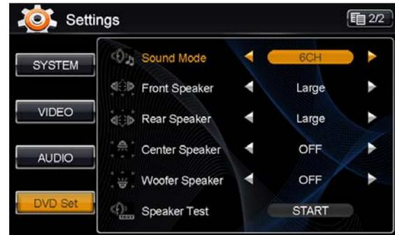
*Note: When Large is selected, the speakers will receive the full frequency spectrum. When Small is selected, the speakers will only receive the mid and high frequency.*
