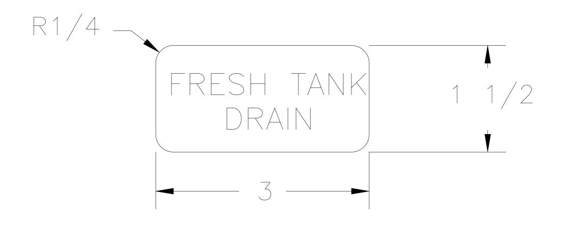
\*LABEL IS ADHESIVE BACKED AND WILL BE LOCATED IN THE BASEMENT STORAGE THAT HOUSES THE LOWER FRESH TANK.
