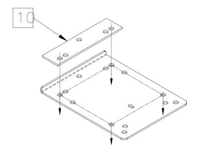
PEDESTAL TO BE MOUNTED TO FLOOR USING THE REARWARD MOST SET OF MOUNTING HOLES THEREBY LOCATING THE SEAT AS FAR FORWARD AS POSSIBLE
