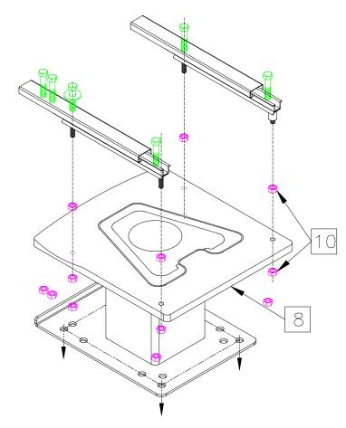
PEDESTAL TO BE MOUNTED TO FLOOR USING THE REARWARD MOST SET OF MOUNTING HOLES THEREBY LOCATING THE SEAT AS FAR FORWARD AS POSSIBLE
