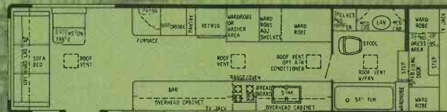
40' WALK THRU FRONT BATH - DRY WT. 9200 lbs. - HITCH WT. 2000 lbs. - OVERALL LENGTH 39' 7"
