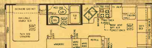
29' CENTER BATH T.T. - DRY WT. 6500 lbs. - HITCH WT. 850 lbs. - OVERALL LENGTH 29' 5-1/2"
