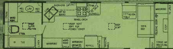
35' REAR BATH PLAN #1 - DRY WT. 8200 lbs. - HITCH WT. 1650 lbs. - OVERALL LENGTH 35' 4"
