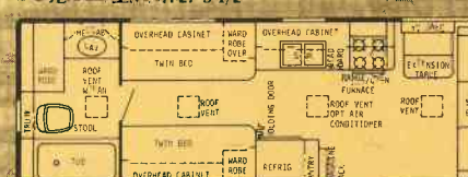
27' REAR BATH T.T. - DRY WT. 5800 lbs. - HITCH WT. 650 lbs. - OVERALL LENGTH 27' 5-1/2"
