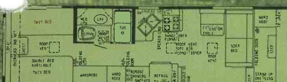
35' CENTER BATH - DRY WT. 8200 lbs. - HITCH WT. 1650 lbs. - OVERALL LENGTH 35' 4"
