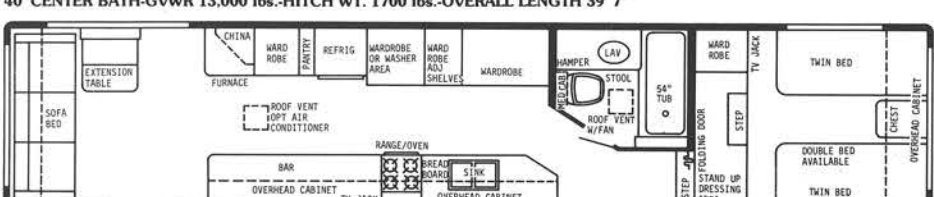
40' FRONT BATH DOORSIDE KITCHEN-GVWR 13,000 lbs.-HITCH WT. 2000 lbs.-OVERALL LENGTH 39' 7"
