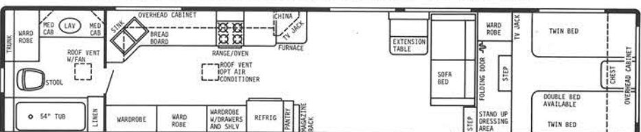
40' REAR BATH PLAN #2-GVWR 13,000 lbs.-HITCH WT. 1700 lbs.-OVERALL LENGTH 39' 7"
