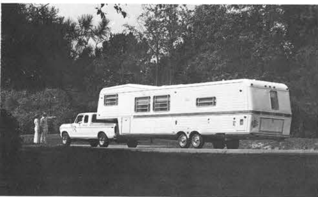
28' FRONT BATH DOORSIDE KITCHEN-GVWR 10,000 lbs. - HITCH WT. 1800 lbs.-OVERALL LENGTH 28' 7-1/2"
