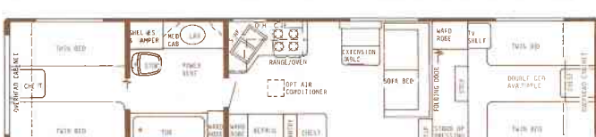
35' Walk-Thru Center Bath - Dry Wt. 8500 lbs. - Hitch Wt. 1650 lbs. - Overall Length 35'6"
