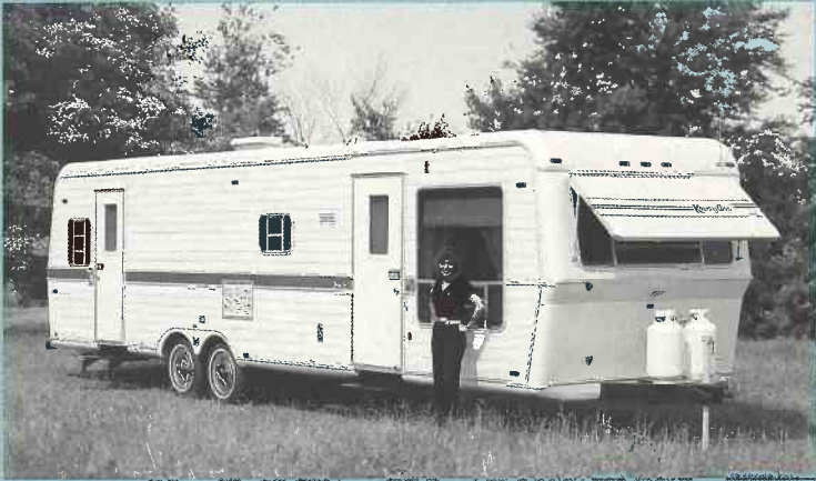
27' Rear Bath - Dry Wt. 5900 lbs. - Hitch Wt. 550 lbs. - Overall Length 27'5"
