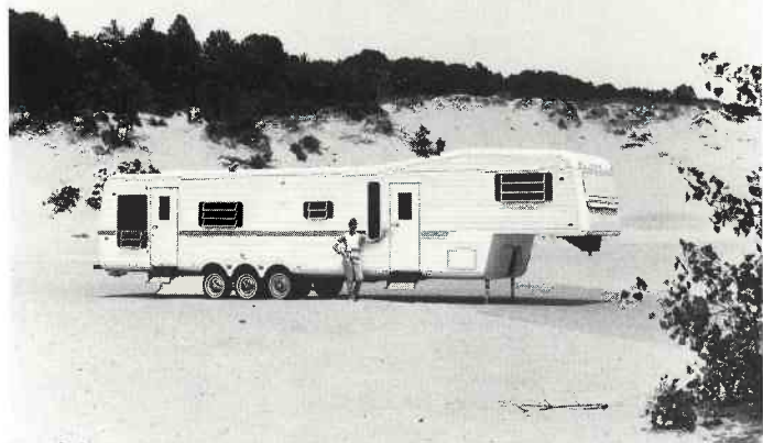
32' Front Bath Doorside Kitchen - Dry Wt. 7500 lbs. - Hitch Wt. 1650 lbs. - Overall Length 32'6"
