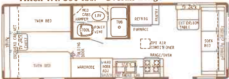
27' Center Bath - Dry Wt. 5900 lbs. - Hitch Wt. 550 lbs. - Overall Length 27'5"
