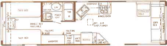
33' Center Bath - Dry Wt. 6900 lbs. - Hitch Wt. 700 lbs. - Overall Length 33'5"
