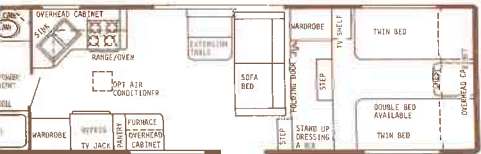
35' Bath - Dry Wt. 6600 lbs. - Hitch Wt. 1650 lbs. - Overall Length 28'8"
