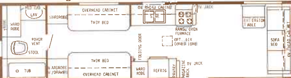
33' Rear Bath - Dry Wt. 6900 lbs. - Hitch Wt. 700 lbs. - Overall Length 33'5"
