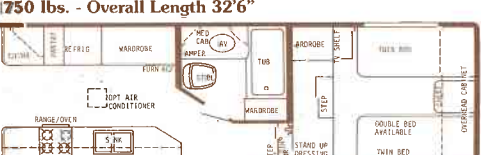
35' Doorside Kitchen - Dry Wt. 7500 lbs. - Hitch Wt. 1750 lbs. - Overall Length 32'6"
