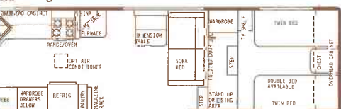
35' Dry Wt. 7500 lbs. - Hitch Wt. 1750 lbs. - Overall Length 32'6"
