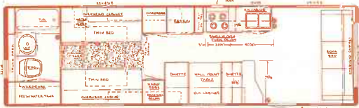
31' Rear Bath Dinette Travel Trailer Dry Weight - 5200 lbs. Hitch Weight - 500 lbs. Overall Length - 30' 11"
