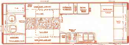
27' Rear Bath Travel Trailer Dry Weight - 4400 lbs. Hitch Weight - 500 lbs. Overall Length - 26' 11"
