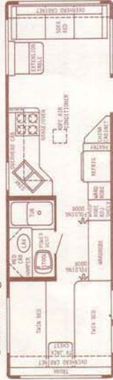
31' Rear Bath - Dry Wt. 6700 lbs. - Hitch Wt. 700 lbs. - Overall Length 31'5"
