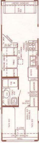
33' Rear Bath - Dry Wt. 6900 lbs. - Hitch Wt. 700 lbs. - Overall Length 33'5"
