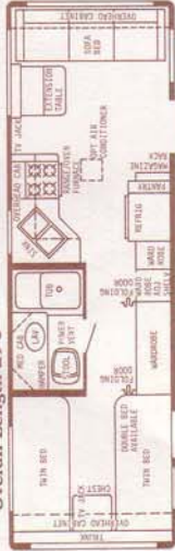
29' Rear Bath - Dry Wt. 6500 lbs. - Hitch Wt. 675 lbs. - Overall Length 29'5"
