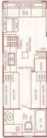
27' Rear Bath - Dry Wt. 5900 lbs. - Hitch Wt. 550 lbs. - Overall Length 27'5"
