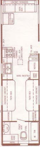
33' Center Bath - Dry Wt. 6900 lbs. - Hitch Wt. 700 lbs. - Overall Length 33'5"
