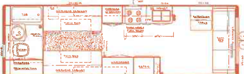
29' Rear Bath Travel Trailer Dry Weight - 4800 lbs. Hitch Weight - 500 lbs. Overall Length - 28' 11"
