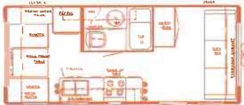
22' Center Bath Travel Trailer Dry Weight - 3600 lbs. Hitch Weight - 400 lbs. Overall Length - 21' 11"
