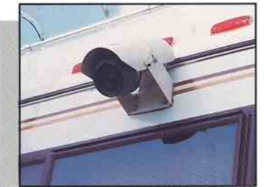
Closed-circuit rear view monitor (standard) makes maneuvering easier in the Class A.
