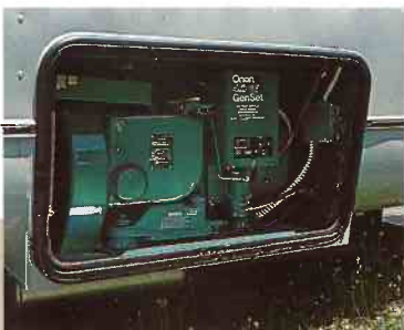
ONAN 110V, 4000W generator.
