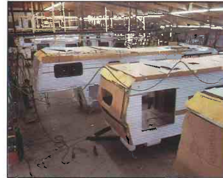
Roof lines are aerodynamically rounded to reduce wind resistance.
