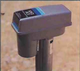
12 volt Electric Tongue Jack, standard on London Aire Travel Trailers.
