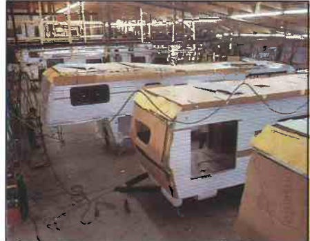
Roof lines are aerodynamically rounded to reduce wind resistance.
