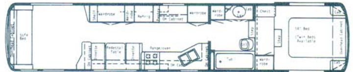
(4) 40 Front Bath Doorside Kitchen • Overall Length 40' 0"
