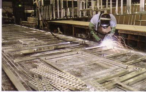
The welded aluminum sidewall construction is built with 16" on center framing, providing the strongest and most durable construction possible.
