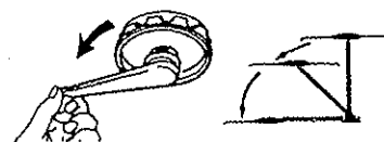
LOWERING ANTENNA TO TRAVEL POSITION
