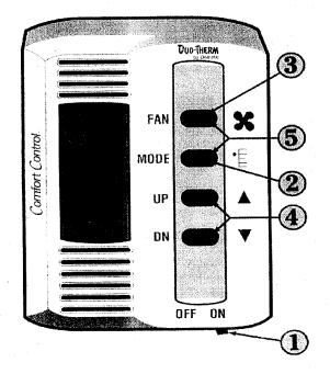
**Shutdown:** If you turn the Comfort Control off or if there is a power interruption for any reason, the system will resume operation on the last settings when power returns.
