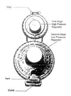
The presence of moisture in LP fuel causes the regulators to freeze. The moisture will pass through the cylinder valve and into the regulator where freezing occurs. To help prevent the regulator from freezing, always keep the tank control valve closed when not in use, even when the tank is empty, to prevent moisture from collecting on the inside.
