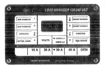
is required. For example, since this unit is equipped with a 50-amp service, it can operate when connected to a shore power source with either a 30-, 20- or 15-amp service.
