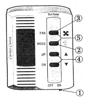
**Shutdown:** If you turn the Comfort Control off or if there is a power interruption for any reason, the system will resume operation on the last settings when power returns.
