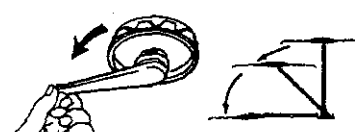
LOWERING ANTENNA TO TRAVEL POSITION
