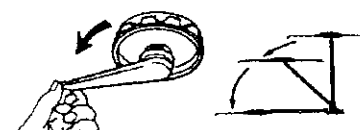
LOWERING ANTENNA TO TRAVEL POSITION
