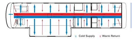
TRUE CENTRAL AIR: Newmar's True Central Air Systemstandard with every Newmar RV-is just like those found in most site-built homes. It's actually two separate, fully ducted systems: one to distribute incoming cool air, the other to quickly and effectively remove warm air from every living area.
