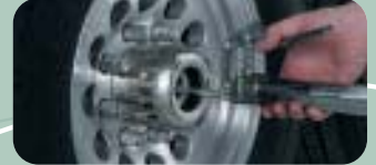
EZ Lube® axles allow RVers to periodically lubricate the bearings without removing hubs from the axles. (Shown with optional polished aluminum wheels.)
