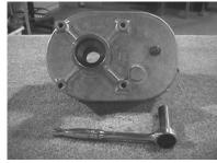
2. Using a 1/2" drive – 11/2" open end wrench and a 1/2" drive ratchet wrench, loosen the 11/2" nut. This will require approximately 11/2 turns. The nut is a standard right hand thread. After the initial release, the nut will turn for a partial turn, and then will release again as you turn the wrench. This second release is required to loosen the TRANS-TORQUE bushing from the shaft.
