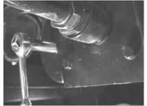
using the hex nut, the room can also be extended or retracted by using the procedure described for the shaft end- mounted motors. If the room is moved using this method, the correct torque on the 11/2" trans-torque nut is 125 foot pounds maximum.
