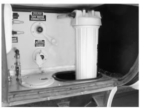
To replace the filter cartridge, turn off the water supply to the RV (at the city water connection). Unscrew the filter canister by rotating it clockwise.
