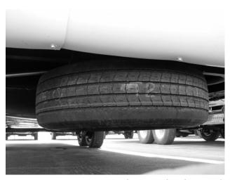
and crank the tire down, or up as necessary. Be sure the spare time is securely positioned for travel, and regularly check the air pressure in the tire to be certain it is ready for use at all times.
