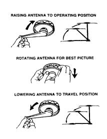
improved. The antenna must be lowered before moving the vehicle. To lower, rotate the directional handle until the pointer is aligned with the pointer on the ceiling plate. Turn the elevating crank (counter-clockwise) in the "DOWN" direction, about 13 turns, or until some resistance to turning is noticed. The antenna is now locked and in the travel position. Your unit may be equipped with one exterior antenna jack and two interior antenna jacks.
