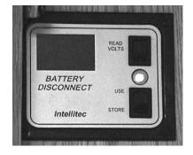
disconnects all of the 12 volt circuitry from the house batteries, with the exception of the LP detector. When taking the unit out of storage, press upward to re-connect the batteries. This will make the 12 volt system ready for use.
