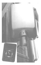
The side exterior mirrors are adjusted by using the multiple directional switch located on the driver's door. Select the mirror to be adjusted by pointing the arrow in the direction of that mirror. Move the control in the direction of movement desired to obtain the best view. The adjustment control moves the top half of both mirrors. The bottom half of the mirror is convex and is adjusted manually. These mirrors also contain heating
