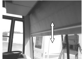
When ready to retract it, tug it gently but firmly down to release the integral catch mechanism, and hold bottom of the screen as the spring tension in the roller retracts it back into it's stored position. Do not release it and allow it to retract rapidly as damage may occur.
