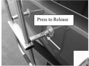
When raised, the hinges have a slotted feature that allows you to rest the lower portion of the ladder in an upright position for access to the engine bay.
