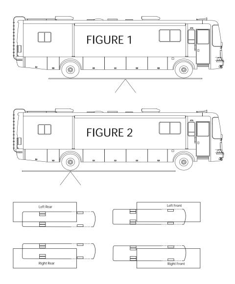
The recommended procedure to weigh a motorhome accurately is on individual corner scales. Since these are not always available, below is a diagram of how to weigh a motorhome on a typical truck scale.
