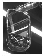
desired to obtain the best view. The adjustment control moves the top half of both mirrors. The bottom half of the mirror is convex and is adjusted manually. These mirrors also contain heating elements to defog or de-ice the mirror glass during cold weather operation. The ON/OFF switch for this feature is located by the adjustment control. The convex exterior chrome mirrors with remote control and defrost are optional on this unit.
