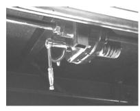
2. Using a 1/2" drive – 11/2" open end wrench and a 1/2" drive ratchet wrench, loosen the 11/2" nut. This will require approximately 11/2 turns. The nut is a standard right hand thread. After the initial release, the nut will turn for a partial turn, and then will release again as you turn the wrench. This second release is required to loosen the TRANS-TORQUE bushing from the shaft.
