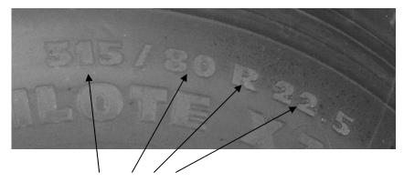
This tire size is 315 / 80 R 22.5. From this size, we can determine the physical dimensions of the tire, as well as it's basic construction. The tire size breaks down like this:
