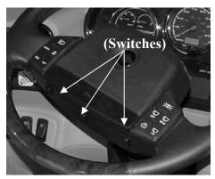
to position the wheel for comfort and an excellent view of the instruments. The center switch allows the driver to telescope the steering wheel position in or out, again to provide for greater comfort and an unimpaired view of the gauges.
