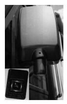
The adjustment control moves the top half of both mirrors. The bottom half of the mirror is convex and is adjusted manually. These mirrors also contain heating elements to defog or de-ice the mirror glass during cold weather operation. The ON/OFF switch for this feature is located by the adjustment control. The convex exterior chrome mirrors with remote control and defrost are optional on this unit.
