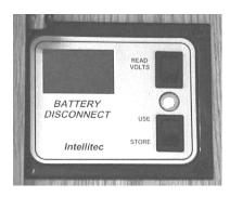
This is done to prevent the coach batteries from being drained during storage. It disconnects all of the 12 volt circuitry from the batteries, with the exception of the LP detector. When taking the unit out of storage, press upward to reconnect the batteries. This will make the 12 volt system ready for use.
