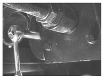
After the initial release, the nut will turn for a partial turn, and then will release again as you turn the wrench. This second release is required to loosen the TRANS-TORQUE bushing from the shaft.
