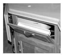
Metal drawer guides are installed on the drawers in your unit. These guides provide a smooth opening and closing of the drawers. To open a drawer, lift up slightly and pull open. The way this mechanism works will prevent the drawers from unintended opening while traveling.
