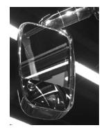
feature is located by the adjustment control. The convex exterior chrome mirrors with remote control and defrost are optional on this unit.
