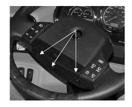
(on the left) tilts the steering column up and down to allow for easy access to the drivers seat, while still allowing the driver to position the wheel for comfort and an excellent view of the instruments. The center switch allows the driver to telescope the steering wheel position in or out, again to provide for greater comfort and an unimpaired view of the gauges.
