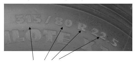
This tire size is 315/80 R 22.5. From this size, we can determine the physical dimensions of the tire, as well as it's basic construction. The tire size breaks down like this:
