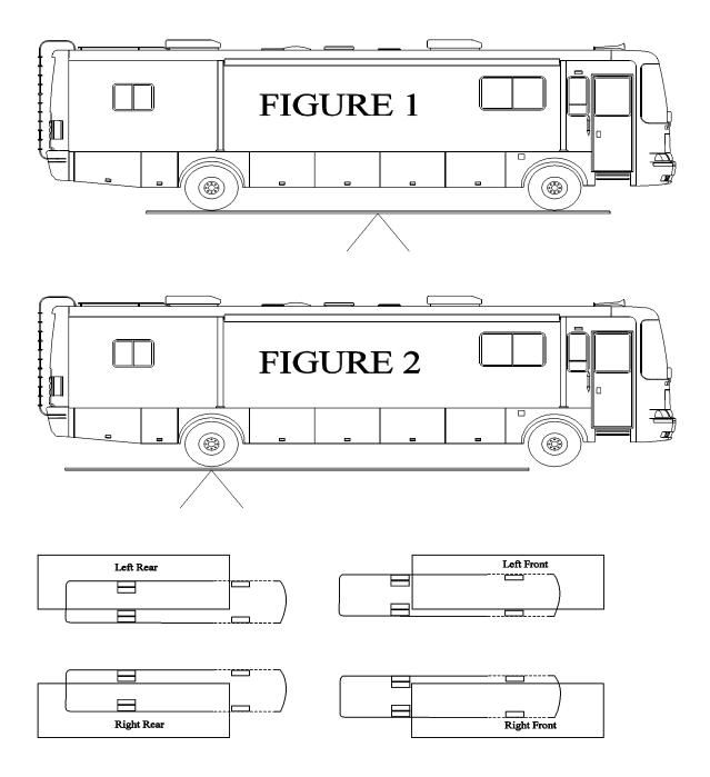
The recommended procedure to weigh a motorhome accurately is on individual corner scales. Since these are not always available, below is a diagram of how to weigh a motorhome on a typical truck scale.
