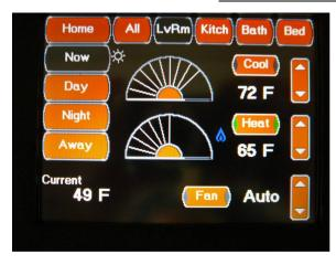
The Climate "LvRm" Screen displays the Heating and Cooling controls for Living Room zone.
