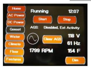
The Genset Screen displays the current Generator Status. The Start and Stop Buttons allow you to manually start and stop the generator. The Clear AGS Button allows you to clear the AGS Safety Lockout flag to reset the Auto Gen function..
