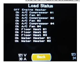
The Load Status Screen displays the electrical status of all the AC powered devices that are controlled by the control system. This screen also displays the AC voltage and amperage usage on both power legs
