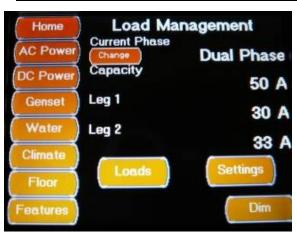
The Load Management Screen displays the Shore Power Phase setting (Single Phase 30 Amps and less Service, Dual Phase 50 Amp Service) and allows you to change between the phase selections using the Change Button. The current Amp draw is displayed for both legs on this screen. The Load Status screen is selected from the Loads Button. The Load Settings Screen is selected from the Settings Button.
