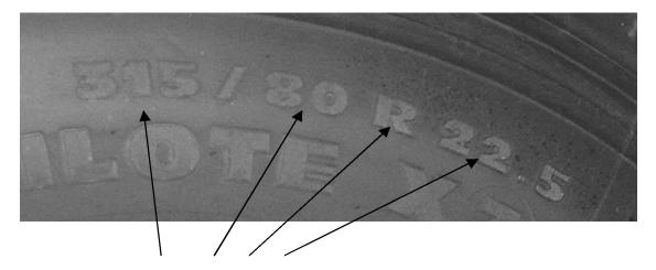
This tire size is 315 / 80 R 22.5. From this size, we can determine the physical dimensions of the tire, as well as its basic construction. The tire size breaks down like this:
