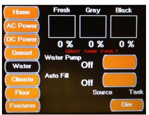
The Water Screen on coaches equipped with the All Electric option displays the Fresh and Holding Tanks volume % full status. This screen also displays tank related faults, if any. The Water Pump Button turns the Water Pump on and off. The Auto Fill Button turns the Auto Fill function on and off.
