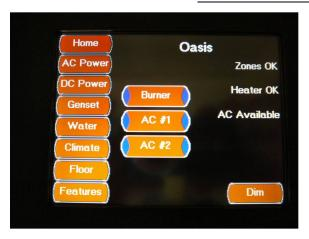
The Oasis Screen is accessed from the Oasis Button displayed in the Climate All Screen. This screen controls the Oasis Burner and both AC Heating Elements. The Burner, AC #1 and AC #2 Buttons will highlight when active. This screen also displays the Oasis System operational Status and Faults.
