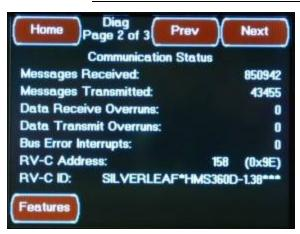
This second Systems Diagnostics Screen is accessed by pressing the Next Button located on the first Systems Diagnostics Screen or from the "Prev" Button located on third Systems Diagnostics Screen. This Screen displays communications status present on the control system.
