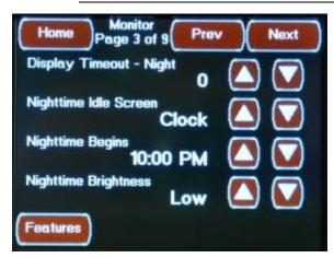
This third Monitor Configuration Screen is accessed by pressing the Next Button located on the second Monitor Configuration Screen or from the "Prev" Button located on fourth Monitor Configuration Screen. This Screen allows you to set the Night Time Display Settings by pressing the associated Up and Down Buttons.
