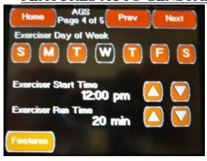
This fourth Autogen Configuration screen is accessed by pressing the Next Button located on the third Autogen Configuration screen or by pressing the "Prev" Button located on the fifth Autogen Configuration screen. This screen allows you to change the following settings:
