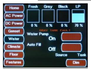
The Water Screen for a coach equipped with a LP tank displays and controls the same functions as the All Electric Water Screen with the addition of the LP tank fill status.
