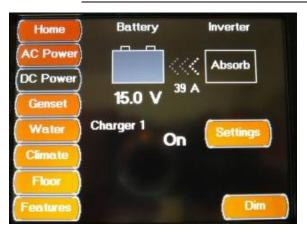
The Main DC Power Screen displays the Inverter / Charger status and allows access to the Magnum Setting Screens
