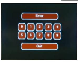
The Password Access Screen is displayed to provide access to advanced system configuration screens. The advanced configuration screens contain control settings that should only be changed by qualified individuals. Changing these control settings to an improper setting can adversely affect the operation of the control system and may cause damage to the coach.
