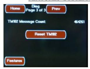
This third Systems Diagnostics Screen is accessed by pressing the Next Button located on the second Systems Diagnostics Screen. This Screen displays additional communications status present on the control system.
