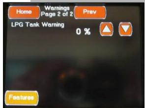
This second Warnings Configuration screen is accessed by pressing the Next Button located on the first Warnings Configuration screen. This screen allows you to change the following settings:
