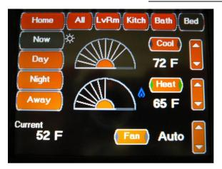
The Climate "Bed" Screen displays the Heating controls for Bedroom zone.
