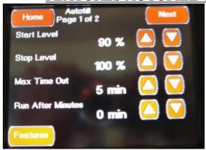
This first Autofill Configuration screen is accessed by pressing the Autofill Configuration
