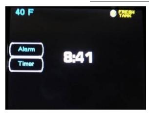
This screen is accesses by pressing the Clock Button form The Features Screen. This screen displays the system time and allows you to access both the Alarm Clock and Countdown Timer functions.
