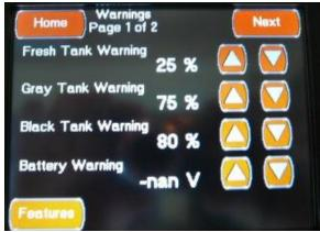
This first Warnings Configuration screen is accessed by pressing the Warnings Configuration Button located on the Features Configuration Screen or by pressing the "Prev" Button located on the second Warnings Configuration screen. This screen allows you to change the following settings:
