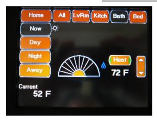
The Climate "Bath" Screen displays the Heating controls for Bathroom zone. Since the Bathroom does not have an air conditioner there is no Cool Button displayed on this screen.
