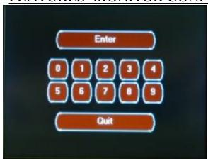
The Password Access Screen is to provide access to advanced system configuration screens. These screens contain control settings that should only be changed by qualified individuals.
