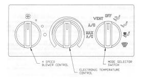
The Passenger Control Panel enables the passenger to the temperature and volume (speed) of the air being discharged to the passenger side of the vehicle.
