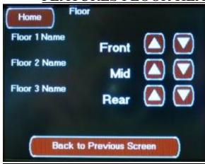
This Floor Heat Configuration Screen is accessed by pressing the Floor Heat Configuration Button located on the Features Configuration Screen. This screen is only available on systems with the Floor Heat option. This screen allows you to change the following settings:
