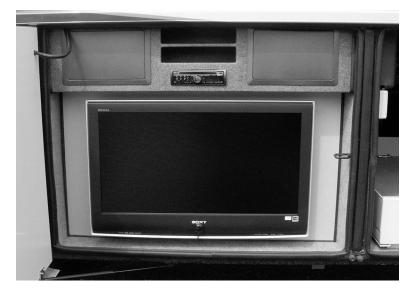
release and swing freely to the desired viewing position. To store the TV for travel, swing it back into the opening, taking that it is fully latched.
