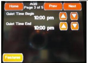
This third Autogen Configuration screen is accessed by pressing the Next Button located on the second Autogen Configuration screen or by pressing the "Prev" Button located on the fourth Autogen Configuration screen. This screen allows you to change the following settings:
