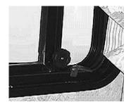
A 12 volt vent may be installed in the kitchen. This vent is equipped with a rain sensor on the roof hood. Anytime the vent is open and it senses rain, it will automatically close. The vent is controlled by the wall switch. Do not leave the fan in active mode while the unit is in storage or unattended for long periods of time. High winds or other unusual conditions or obstructions may prevent the vent from closing resulting in leakage, which could cause serious damage.
