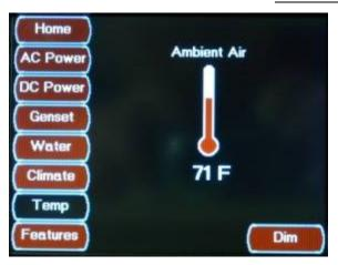
The Temp screen is accessed by pressing the Temp Button located on the Home Screen. This screen displays the Outside Air Temperature and only exists on systems without the optional Floor Heat.
