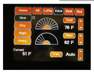
The Climate "Kitch" Screen displays the Heating and Cooling controls for Kitchen zone.
