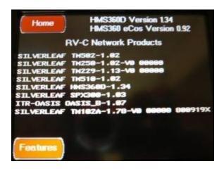
This Component Versions screen is accessed by pressing the Components Versions Button located on the Features Configuration Screen. This screen displays all of the RV-C Modules and their firmware versions found on the system.
