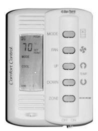
Step One: Move power switch to ON.
