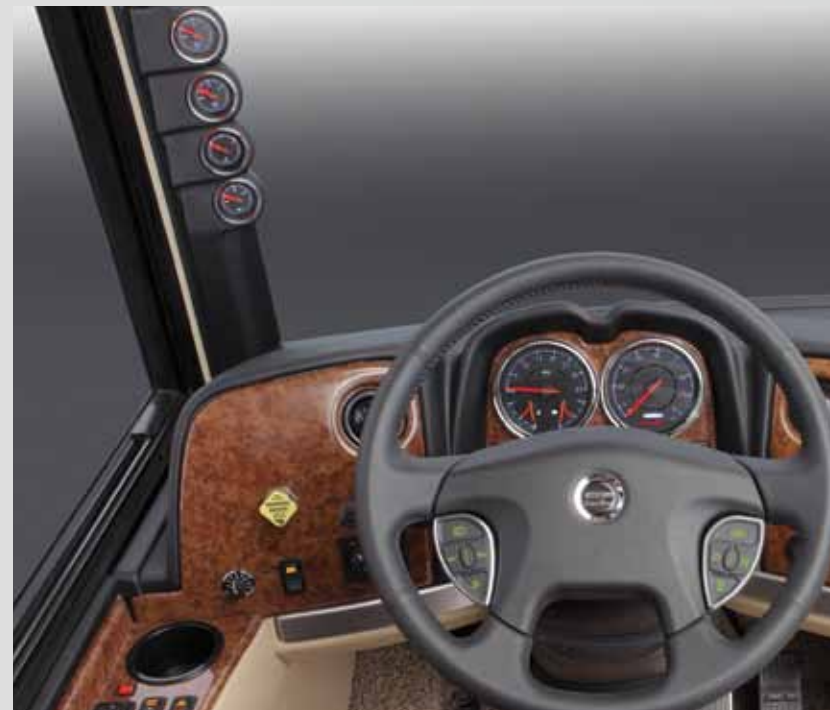
STACKED, LINE OF SIGHT GAUGE STRUCTURE
