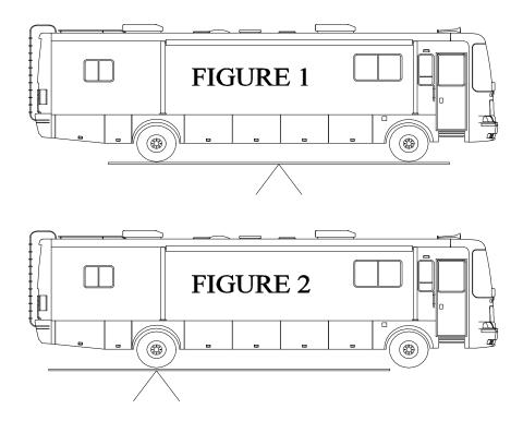
The recommended procedure to weigh a motorhome accurately is on individual corner scales. Since these are not always available, below is a diagram of how to weigh a motorhome on a typical truck scale.
