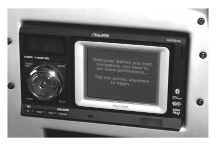
Your Ventana may be equipped with an Eclipse stereo radio, featuring a removable Navigation screen. This allows you to use the TomTom GPS system in multiple vehicles. For complete operating details, please refer to the manufacturer's literature that is provided in the literature bag for your unit.
