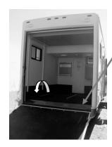
To complete the lowering process, be sure to rotate the hinged ramp cover at the bottom of the door to bridge the gap between the cargo bay floor and the ramp door. This allows for smooth transition as items are loaded up and down the ramp into the cargo bay. Always use caution when loading and unloading cargo.
