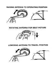
must be lowered before moving the vehicle. To lower, rotate the directional handle until the pointer is aligned with the pointer on the ceiling plate. Turn the elevating crank (counter-clockwise) in the "DOWN" direction, about 13 turns, or until some resistance to turning is noticed. The antenna is now locked and in the travel position. Your unit may be equipped with one exterior antenna jack and two interior antenna jacks.
