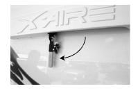
With the trigger pulled, the handle will swing down, releasing the latching mechanism for the rear cargo door (pressing on the door may release some pressure on the latching mechanism to allow the handle to swing down more easily).
