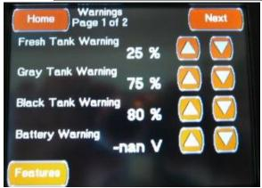
This first Warnings Configuration screen is accessed by pressing the Warnings Configuration Button located on the Features Configuration Screen or by pressing the "Prev" Button located on the second Warnings Configuration screen. This screen allows you to change the following settings:
