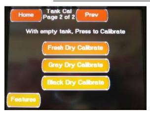
This second Tank Cal screen is accessed by pressing the Next Button located on the first Tank Cal screen.
