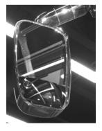
control. The convex exterior chrome mirrors with remote control and defrost are optional on this unit.
