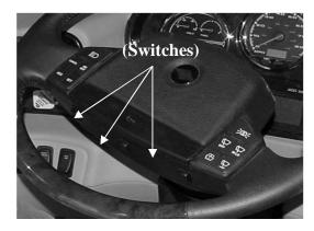
The far right rocker switch moves the brake and throttle pedals under the dash. This allows for greater flexibility in seating position, as well as improved individual access to the pedals.
