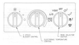
The Main Control Panel enables the driver to control the volume (speed) and temperature of the air for the driver's side of the unit, and the air discharge from the system for both occupants.
