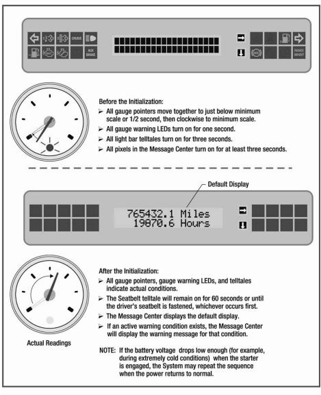
Figure 1-2 System Initialization Sequence
