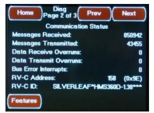
This second Systems Diagnostics Screen is accessed by pressing the Next Button located on the first Systems Diagnostics Screen or from the "Prev" Button located on third Systems Diagnostics Screen. This Screen displays communications status present on the control system.
