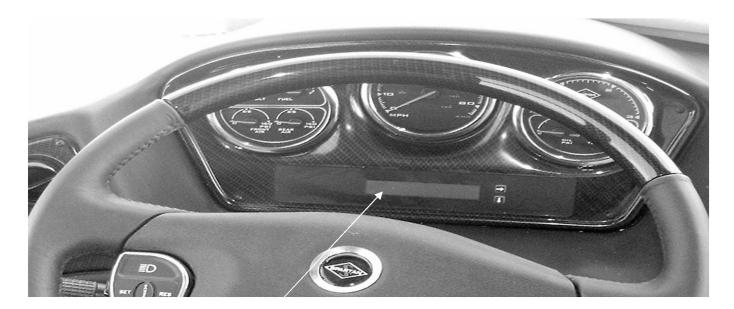
The Spartan Lightbar Message Center is located in the instrument cluster panel, and is designed to provide information to the driver regarding the engine and power train of your King Aire.
