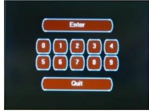
The Password Access Screen is to provide access to advanced system configuration screens. These screens contain control settings that should only be changed by qualified individuals.
