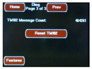
This third Systems Diagnostics Screen is accessed by pressing the Next Button located on the second Systems Diagnostics Screen. This Screen displays additional communications status present on the control system.
