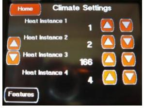
This fifth Climate Setting screen is accessed by pressing the Left Down Arrow on the fourth Climate Setting screen or by the Left Up Arrow on the sixth Climate Setting screen. This screen controls the following:
