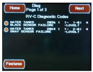
This first Systems Diagnostics Screen is accessed by pressing the System Diagnostic Button located on the Features Screens or from the "Prev" Button located on second Systems Diagnostics Screen. This Screen displays any system faults present on the control system.
