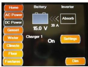
The Main DC Power Screen displays the Inverter / Charger status and allows access to the Magnum Setting Screens
