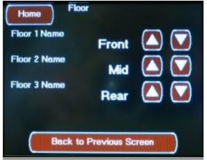
This Floor Heat Configuration Screen is accessed by pressing the Floor Heat Configuration Button located on the Features Configuration Screen. This screen is only available on systems with the Floor Heat option. This screen allows you to change the following settings:
