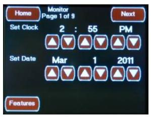
This first Monitor Configuration Screen is accessed by pressing the Monitor Configuration Button located on the Features Screens or from the "Prev" Button located on second Monitor Configuration Screen. This Screen allows you to set the system time and date by pressing the associated up and Down Buttons.
