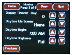
This second Monitor Configuration Screen is accessed by pressing the Next Button located on the first Monitor Configuration Screen or from the "Prev" Button located on third Monitor Configuration Screen. This Screen allows you to set the Day Time Display Settings by pressing the associated Up and Down Buttons.
