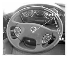
The right side bottom switch moves the brake and throttle pedals under the dash. This allows for greater flexibility in seating position, as well as improved individual access to the pedals.
