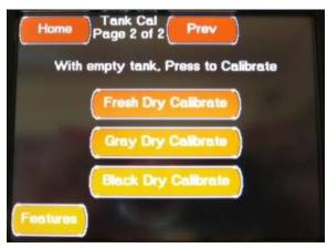
This second Tank Cal screen is accessed by pressing the Next Button located on the first Tank Cal screen.
