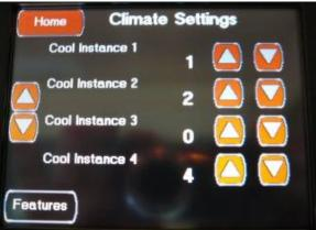
This fourth Climate Setting screen is accessed by pressing the Left Down Arrow on the third Climate Setting screen or by the Left Up Arrow on the fifth Climate Setting screen. This screen controls the following:
