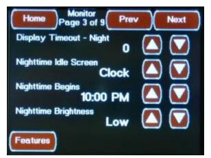
This third Monitor Configuration Screen is accessed by pressing the Next Button located on the second Monitor Configuration Screen or from the "Prev" Button located on fourth Monitor Configuration Screen. This Screen allows you to set the Night Time Display Settings by pressing the associated Up and Down Buttons.
