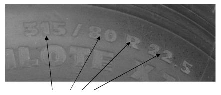
This tire size is 315 / 80 R 22.5. From this size, we can determine the physical dimensions of the tire, as well as its basic construction. The tire size breaks down like this:
