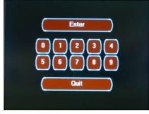
The Password Access Screen is displayed to provide access to advanced system configuration screens. The advanced configuration screens contain control settings that should only be changed by qualified individuals.
