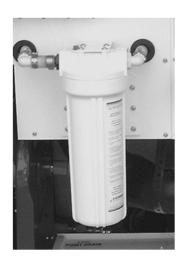
canister. Reattach the canister to the filter housing by rotating the canister in a counter clockwise direction. When replacing the filter, make certain the rubber "O-Ring" seal is properly positioned in its groove in the cartridge housing.
