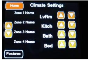
This second Climate Setting screen is accessed by pressing the Left Down Arrow on the first Climate Setting screen or by the Left Up Arrow on the third Climate Setting screen. This screen controls the following:
