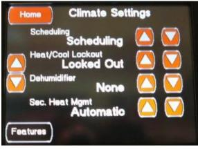
This first Climate Setting screen is accessed by pressing the Climate Configuration Button located on the Features Configuration Screen or by pressing the Left Up Arrow located on the second Climate Setting screen. This screen allows you to change the following settings:
