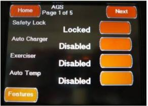
This first Autogen Configuration screen is accessed by pressing the Autogen Configuration Button located on the Features Configuration Screen or by pressing the "Prev" Button located on the second Autogen Configuration screen. This screen allows you to change the following settings: i Safety Lock Select using the Up / Down Arrows
