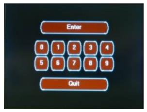
The Password Access Screen is displayed to provide access to advanced system configuration screens. The advanced configuration screens contain control settings that should only be changed by qualified individuals. Changing these control settings to an improper setting can adversely affect the operation of the control system and may cause damage to the coach.
