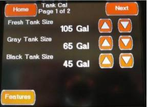
This first Tank Cal screen is accessed by pressing the Tank Calibration Button located on the Features Configuration Screen or by pressing the "Prev" Button located on the second Tank Cal screen. This screen allows you to change the following settings:
