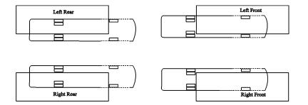
The recommended procedure to weigh a motorhome accurately is on individual corner scales. Since these are not always available, below is a diagram of how to weigh a motorhome on a typical truck scale.
